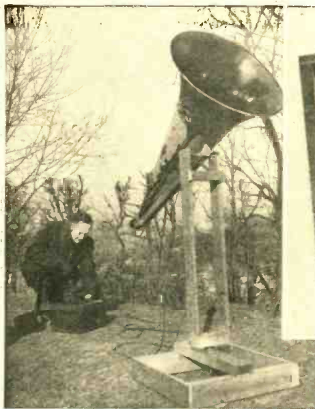
Left—Dr. Donald A. Wilbur of Rensselaer Polytechnic Institute of Troy, New York, tests the airplane sound detector. Above—Interior of the portable amplifier cabinet. Right—Bottom view of amplifier chassis. This airplane detector, made up from an old phonograph horn, mike and battery-operated amplifier, cost about $50 to make.
